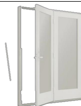
Figure 2c-3 Full Glass French Hinged Door (with center hinges and one door operable)
